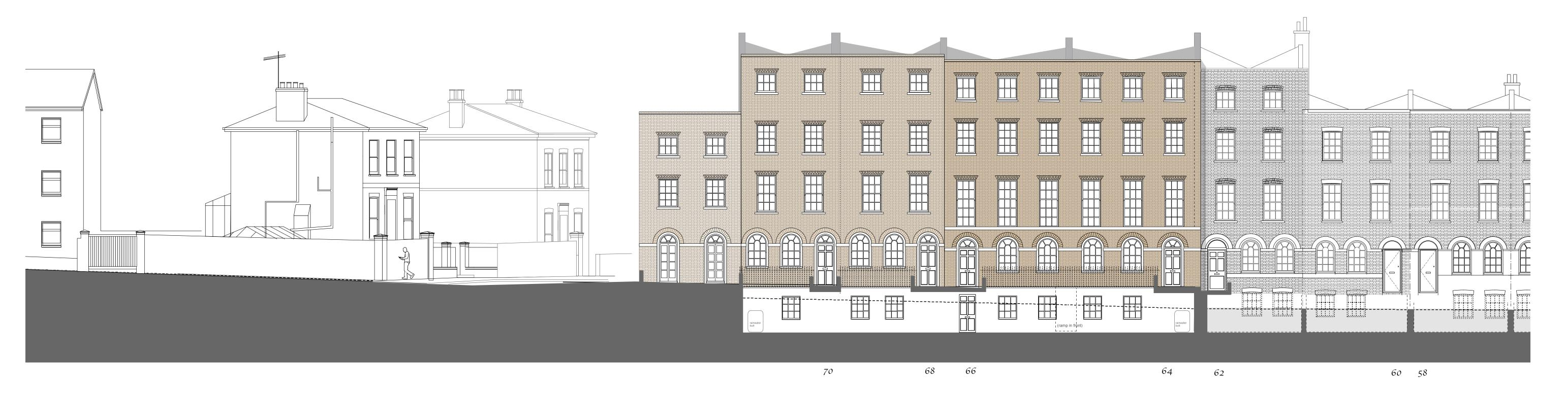
Proposed Front Elevation of Housing, to Grove Lane, showing lower basement areas
